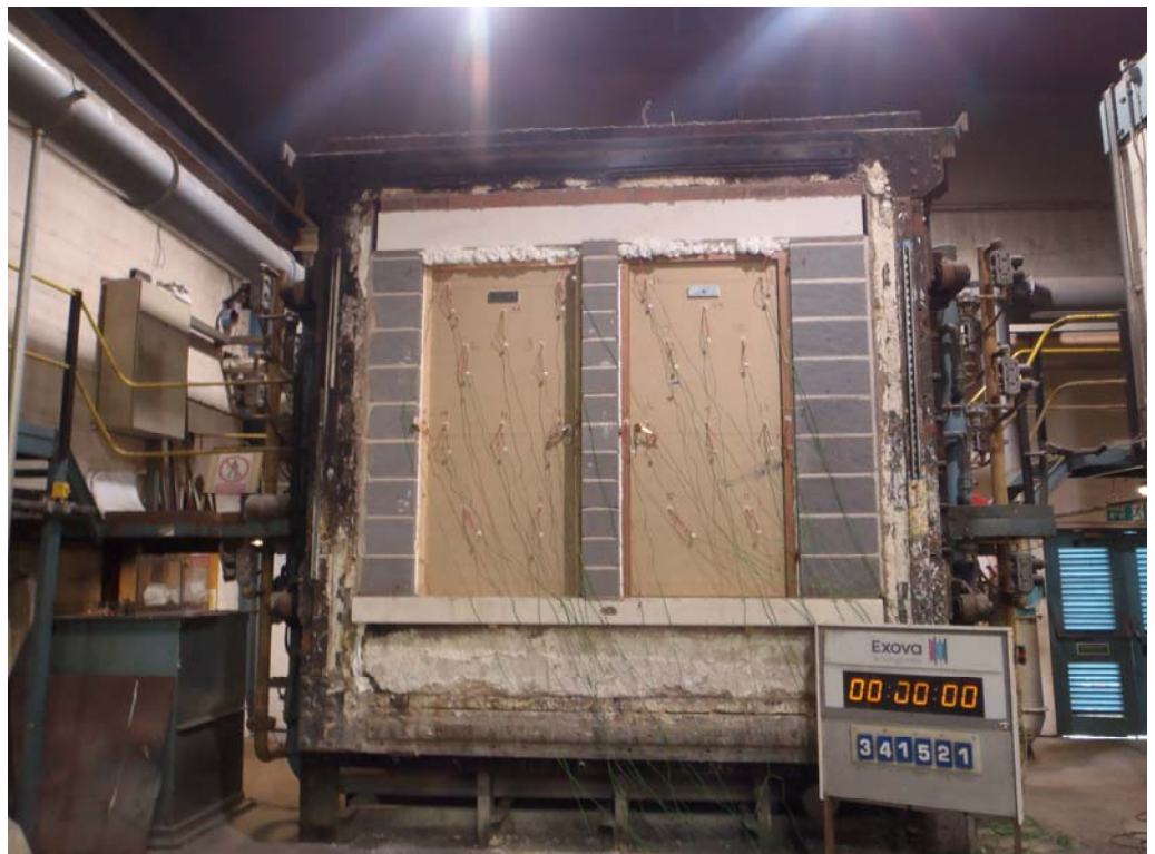
The unexposed face of the doorsets prior to testing
