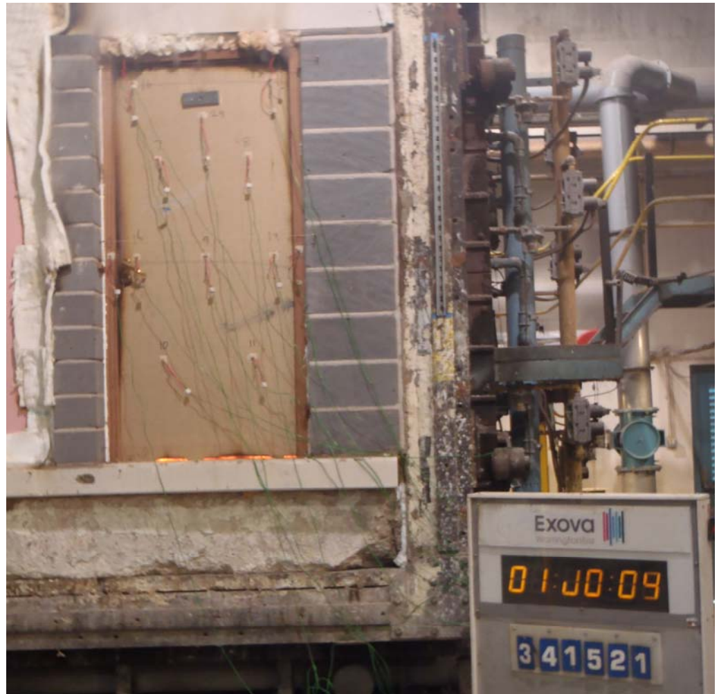
The unexposed face of doorset B after a test duration of 60 minutes
