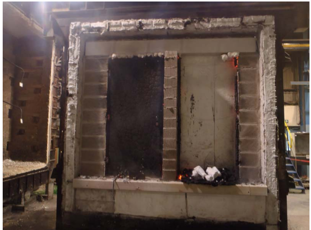
The exposed face of the doorsets after the test.
