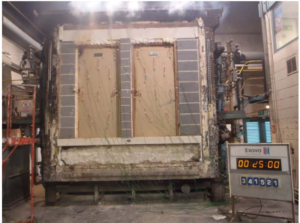
The unexposed face of the doorsets after a test duration of 25 minutes
