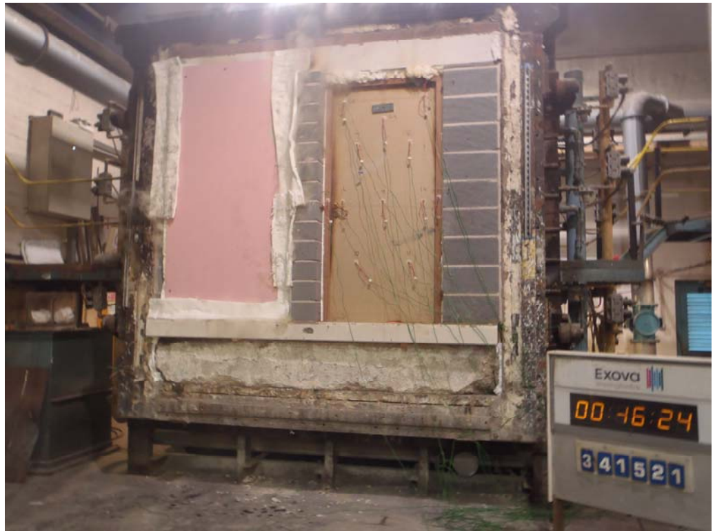
The unexposed face of the doorsets after a test duration of 46 minutes
