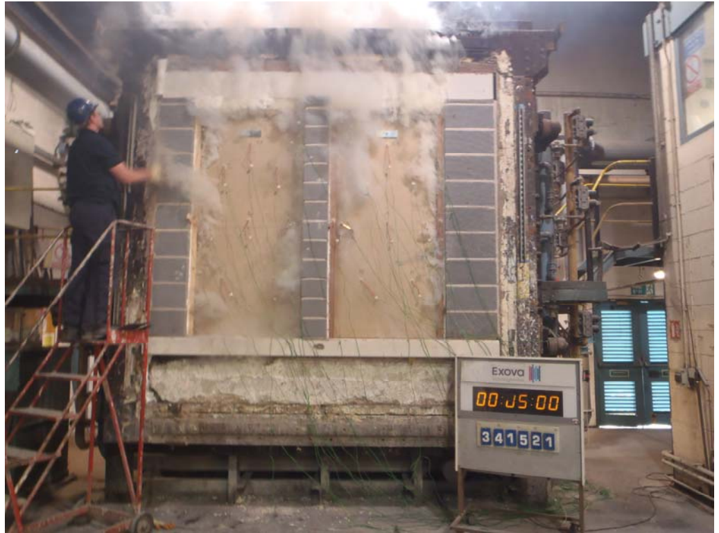
The unexposed face of the doorsets after a test duration of 5 minutes
