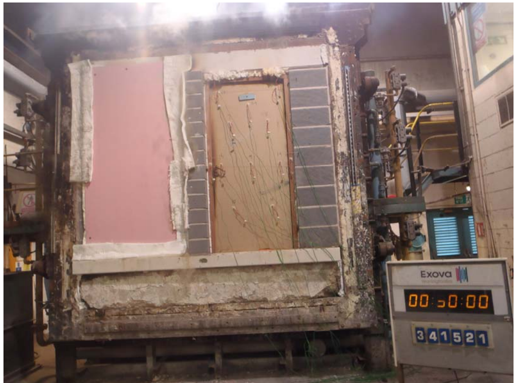
The unexposed face of the doorsets after a test duration of 50 minutes
