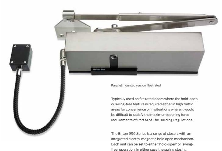
The Briton 996 Series is CE marked to EN 1154 and EN 1155 for electrically controlled closing devices, fire tested to EN 1634 and Certifire Approved for use on timber doors to achieve a 2 hour fire rating.
