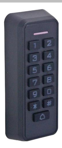
The APX-11 offers the flexibility of a standard keypad with the option to link to a number of mobile phones.
