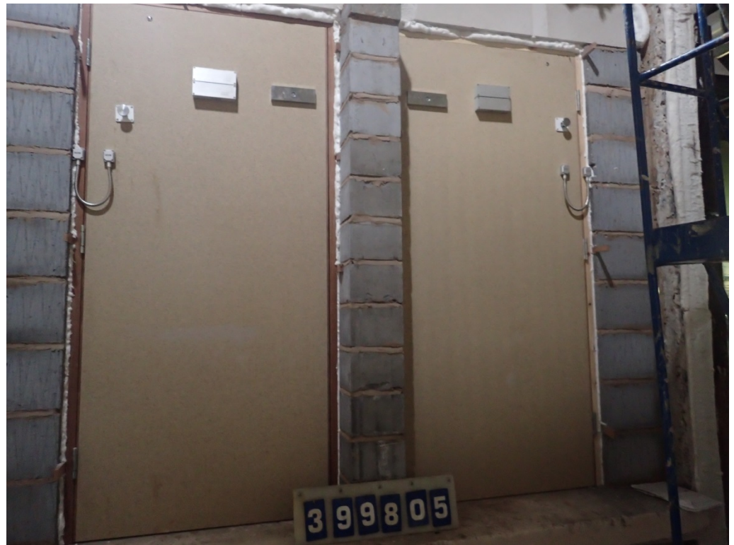
The exposed face of the doorsets prior to testing
