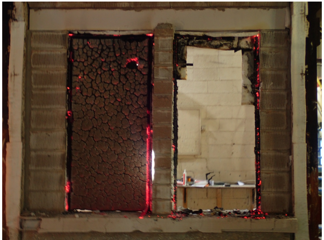
The exposed face of the test assembly immediately after the test
